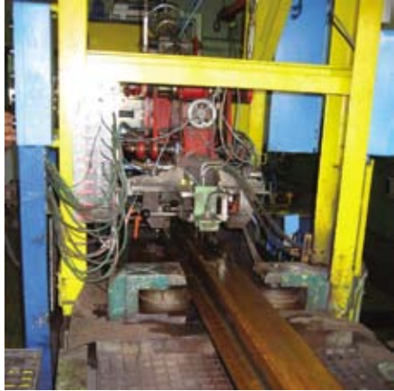
Rail going through the ultra-sonic testing machine.
