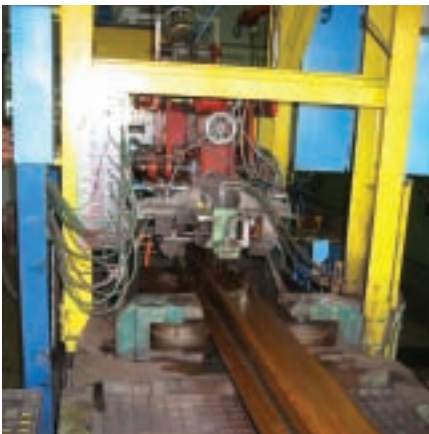
Rail going through the ultra-sonic testing machine.
